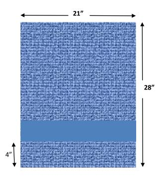
5. Cut two 21" lengths of bias tape. Thread the machine with the all-purpose thread. Attach the edge-joining foot. Select a narrow zig zag, width 2.5mm wide and length 3mm. Position one of the cut bias tape pieces over one of the edges of the contrasting strip, centering the strip over the edge. Position the fabric under the foot, placing the blade of the foot along one of the edges of the bias tape. Stitch in place. Stitch along
