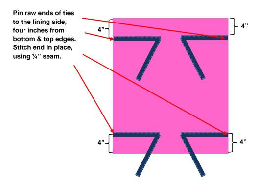
9. Apply remaining bias tape to raw edges of the fabric, enclosing raw edges and mitering the tape at the corners. Stitch in place being careful not to catch tie ends into the seam. Press. Place cover over machine and use ties to secure.
