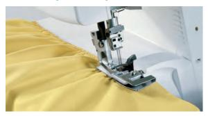
The gathering/ shirring foot is perfect for simultaneously stitching and gathering two layers of fabric, or one layer of fabric. You can increase the gathering by setting a higher differential feed and adjusting the stitch length.
