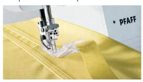
The strap and belt loop Foot is used to create straps and belt loops with a cover stitch. When properly positioned into the strap and Belt Loop Foot L, the bias tape is folded under automatically.
