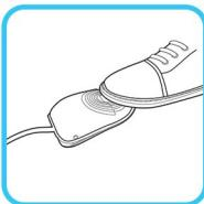
2. To ensure your safety, press the steam pedal until the pressure drops to zero.
