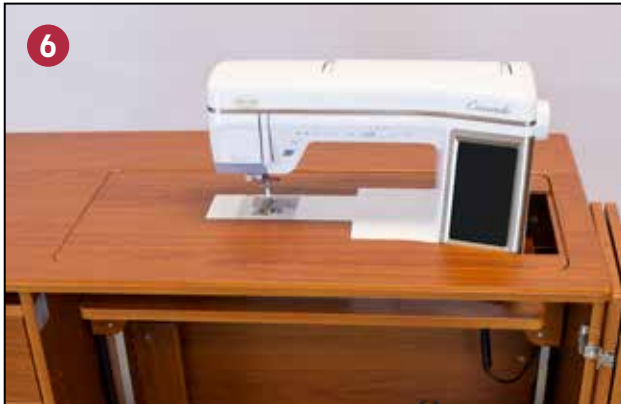
6) This shows the machine positioned level with the Studio top surface with a custom machine insert in place for sewing and quilting. For embroidery and free-arm applications the machine should be positioned at the top level.
