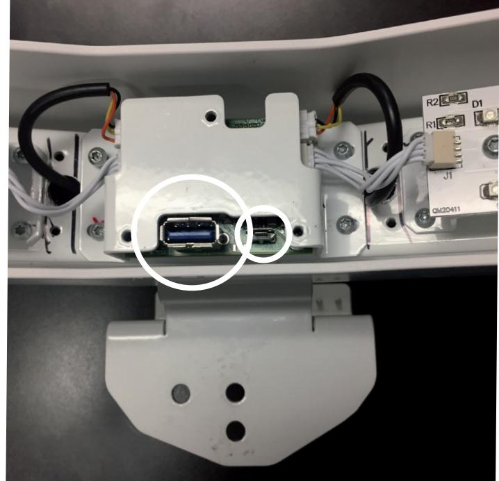
Special Edition front handlebar large USB connection for machine on bottom left and small/micro USB for display on right.
