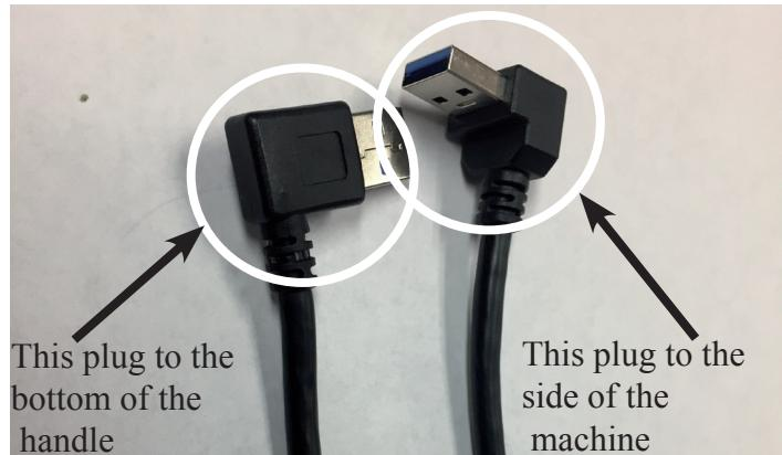
QM23011 Handlebar to machine large USB cable
