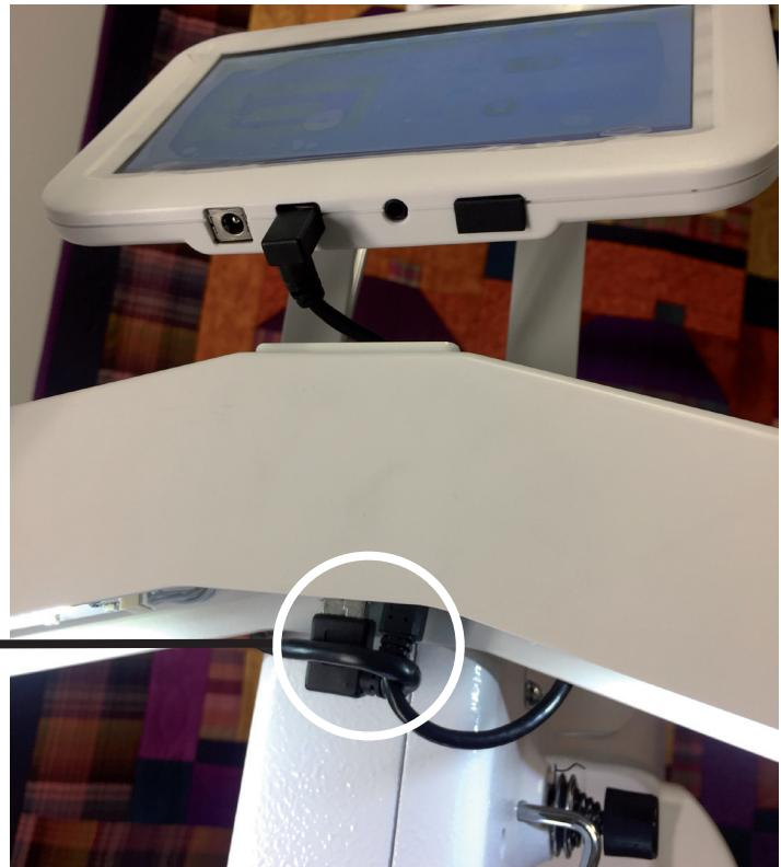
Special Edition front handlebar large USB to machine connection. Note: The bottom right small/micro USB connection above is for the straight small/micro cable end. This connects the handlebar to the display. The display end is a small/micro 90 degree end.
