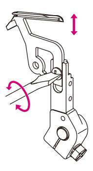
7. ADJUSTMENT OF THE STOPPING POINT OF THE LOWER LOOPER (SYNCHRONIZATION) (USECLAMP).
