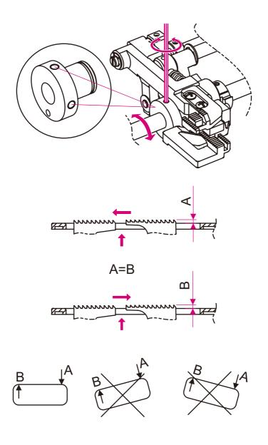
3. ADJUSTMENT OF THE NEEDLE BAR IN RELATION TO THE FEED DOG SHIFT.
