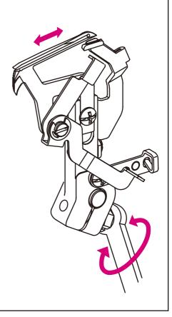
9. CLEARANCE BETWEEN LOWER LOOPER AND THE LEFT AND THE RIGHT HAND NEEDLE.
