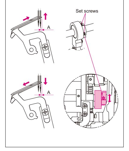
8. CLEARANCE BETWEEN LOWER LOOPER POINT, WHEN AT LEFT MOST POSITION, TO THE LEFT SIDE OF THE LEFT NEEDLE.
