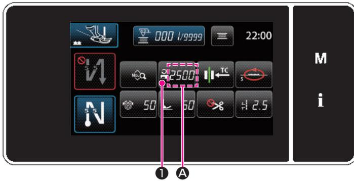
The sewing speed is displayed in section **A** on the panel. (Example of display : 25000 sti/min)
