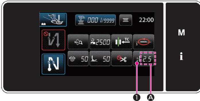
Stitch length is displayed in section **A** on the panel. (Example of display : 2.5 mm)
