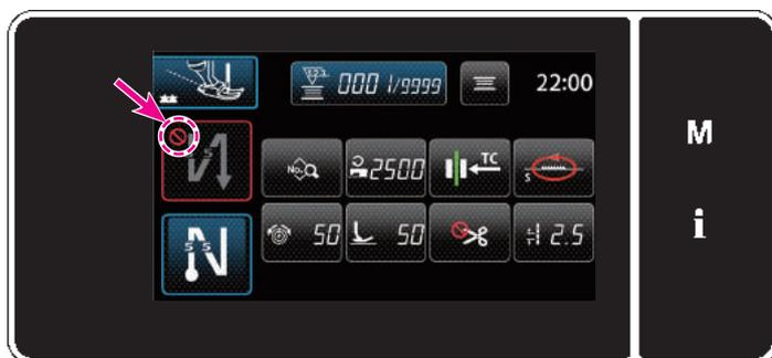
The reverse feed stitching (at start) pattern can be operated when the reverse feed stitching (at start) function is placed in the ON state (⊘ mark is not displayed).
