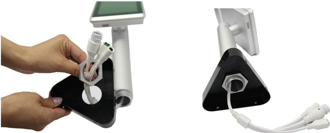
Step 4. Connect the USB, Ethernet, and Power Cable to the Stand Base connectors.
