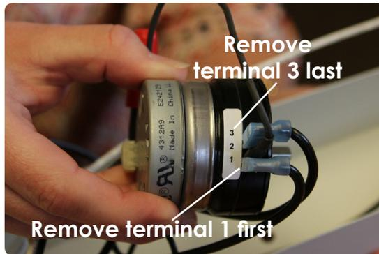
Turn the raceway over so the back is exposed. Lift out the timer and remove the flag shaped connectors from marked terminal 1, and then from marked terminal 3.
