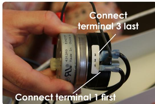
Connect raceway wires to new timer by first connecting long black wire to terminal marked 1. Then connect the shorter wire to terminal marked 3.
