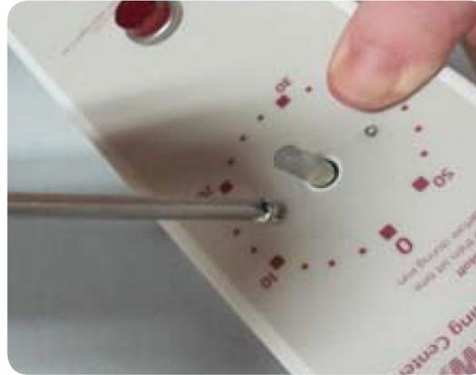
Turn raceway over and screw the two face screws on timer face with Phillips screwdriver. You may need to align screw holes before inserting screws. Replace timer knob on new timer by gently pushing onto shaft of timer.
