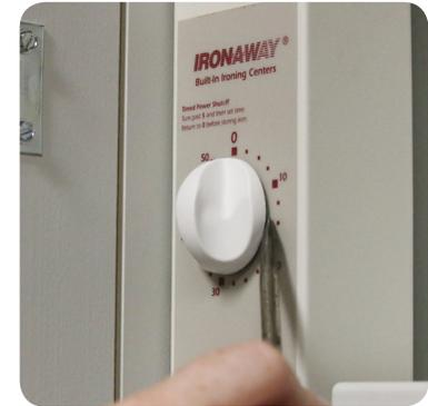
Using a flathead screwdriver, gently pry off the timer knob and lay off to the side.
