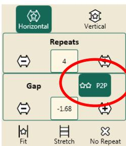
**Note:** P2P snaps the end point of the first design to the start point of the next design.
