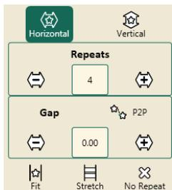
**Note:** Fit will repeat the design at its original size in the area without skewing or stretching.
