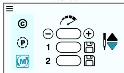
The needle cycles continuously at the same speed, regardless of the movement of the machine.
