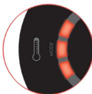
**pureHeat WAVE has a temperature sensor and will enter STANDBY MODE when the temperature in your space has exceeded the set temperature by 2 Degrees. When the Room drops 2 Degrees below the set temperature, the heater will resume normal operation.**
