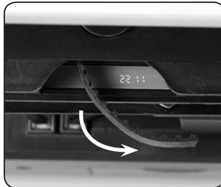
Loop Belt around gear here. **Fig. 7-3**
