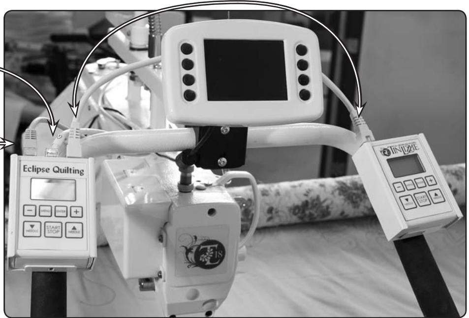
Mounting Eclipse Control box to the Back
