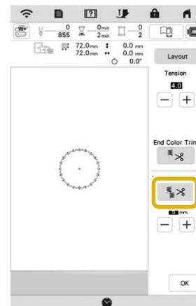
→ The key will display as
