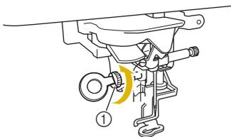
6 Position the embroidery foot “W+” with LED pointer on the presser foot bar by aligning the notch of the presser foot to the large screw.
