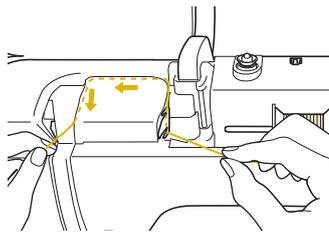
**8** Guide the thread down, up, then down through the groove, as shown in the illustration.
