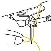
**15** Raise the presser foot lever and pull out about 10 cm (4 inches) of the thread, and then pass it under the presser foot toward the rear of the machine.
