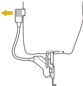
5 Use the included disc-shaped screwdriver to loosen the screw for the embroidery foot, and then remove the embroidery foot “W+” with LED pointer.
