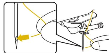
**14** Carefully pull the end of the thread that was passed through the eye of the needle.
