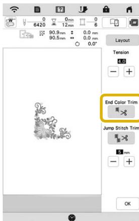
→ The key will display as
