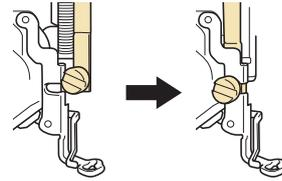
7 Hold the embroidery foot in place with your right hand, and then use the disc-shaped screwdriver to securely tighten the screw for the embroidery foot.
