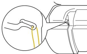
**9** Pass the thread through the needle bar thread guide (marked "6") by holding the thread with both hands and guiding it as shown in the illustration.
