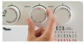
Adjustable Stitch Length and Width - Adjust the length and width for variety or specific techniques like basting or gathering.
