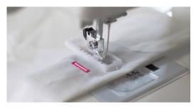
**Four-Step Buttonhole** - With the buttonhole foot, your four-step buttonhole will be sized to match your button every time.
