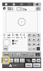
Touch [58] to turn off the thread trimming function.
