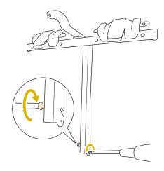
Slide the thread guide assembly support onto the machine, and then tighten the screw, until the thread guide assembly support is secure.
