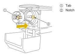
• Fully insert the bobbin case until it snaps into place.
