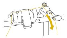
Wind the thread clockwise around the bobbin 4 or 5 times, as shown in the illustration.
