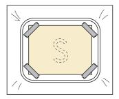
Touch to check the position of the pattern and make sure it does not extend out of the urethane foam. (page 63)
