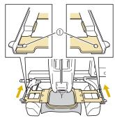
① Make sure that the pins on the left and right arms of the Embroidery Frame Holder fit into the positioning slot and hole on the embroidery frame.
