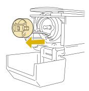
Slide the paper under the tension-adjusting spring to remove any dust.
