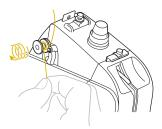
Pass the end of the thread through the guide slit on the bobbin winder seat, and pull the thread. The cutter will cut the thread.
