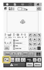
Touch to turn off the automatic thread cutting function.
