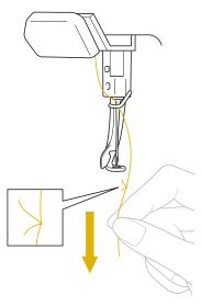
Continue pulling the thread until the knot is below the needle. Cut the knot.
