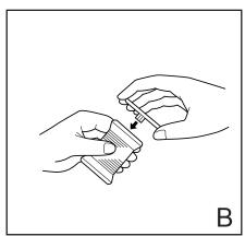
When using standard spool threads on your serger, replace the cone holders with the sponge disks furnished with your machine. These disks hold smaller spools securely and help the thread to reel off properly. With the sponge disk in place, put the capped spool on the spindle. (fig. C)
