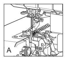
As you sew, you will discover that maneuvering the fabric is different from conventional sewing because the threads form around the stitch fingers. (fig. A)
