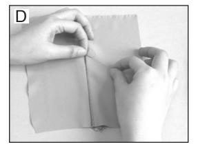
The flatlock stitch need not be limited at seamlines. When sewn on a fold, flatlocking can create attractive decorative effects within the body of a garment or project. Either follow placement lines on your pattern or design your own special effects by stitching the fabric before laying out pattern pieces.
