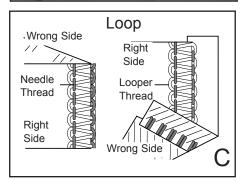
If you want the "overlock stitching" to show on the right side of the fabric, place wrong sides together and sew. (fig. C) To produce the "ladder" (needle thread) on the outside, place the fabric right sides together.
