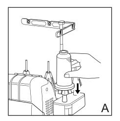
When using threads on cones or king spools, place the cone or spool securely over the cone holders furnished on your machine. To avoid bending the thread stand, you may need to place one hand under the stand while positioning the cone. The cone holders prevent the cone or spool from spinning, enabling the thread to feed evenly. (fig. A)
