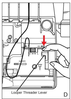
\*Be sure at least 1" of thread is inserted into the threading port.
