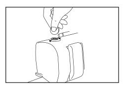
The presser foot pressure has been preset at the factory and rarely needs adjustment. You may find it necessary, however, to decrease the pressure for thick fabrics or increase pressure for thin fabrics to feed more smoothly under the foot. Use a coin to turn the screw on top of the machine.
