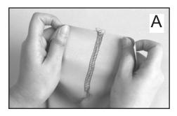
Sew 2-thread flatlock seams in the same way as 3-thread flatlock seams, then pull the two fabric layers apart until the seam lies flat. (fig. A) Because the threads show on the outside as well as the inside of the garment or project, the 2-thread flatlock seam is often considered a decorative application. (fig. B) Be sure to sew a test sample first to determine whether the stitch will have the strength to hold the seam without the fabric pulling away.
