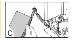
With the needle and upper looper threads under the foot and to the back, lower the presser foot. While holding the threads in your left hand, press down on the foot controller gently to begin a thread chain before serging fabric. (fig. A)
