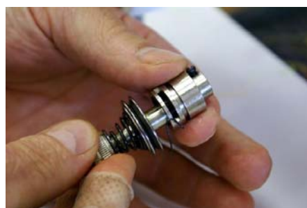
Fig 8: Remove tension assembly from barrel
