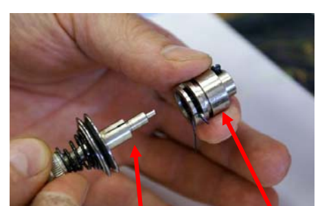
Fig 9: Tension assembly, Barrel
