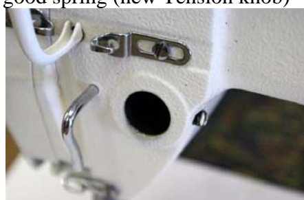
Fig 5: Machine with tension assembly removed
