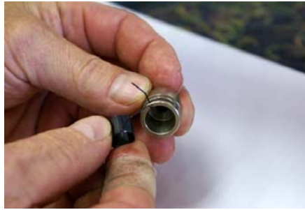
Fig 14: Insert New Spring
