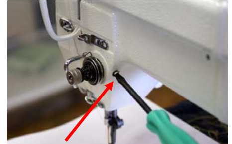
Fig 3: Screw on inside of machine loosen only DO NOT REMOVE
