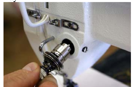
Fig 21: Place the assembly back into your machine
