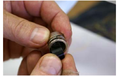
Fig 15: Twist while inserting new spring
