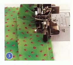
Always test sew a sample first when using the ruffler to make all the adjustments necessary before sewing on your final fabric. If you need to straight stitch you can do so without removing the ruffler attachment. Just move the adjusting lever to the \* position and the ruffler blade will be disengaged.
