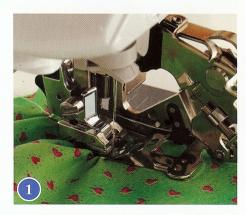
2. To gather and apply to a flat fabric at the same time, with right side down, place the fabric to be gathered in the ruffler as you did in step 1. Place the flat fabric, right side up, under the separator blade on top of the feed dogs. The upper fabric will gather and the bottom fabric will remain flat as you sew. (#2)
