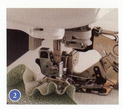
3. You can also gather a double thickness to a flat fabric (e.g. for a ruffle on a pillow). First, cut the ruffle strip and baste the raw edges together. Place the double thickness between the ruffler blade and the separator blade as you have done before. Place the flat fabric under the separator blade on top of the feed dogs. It may be necessary to adjust the depth screw slightly to make sure the fabric is being pushed into the ruffler. (#3)
