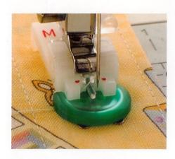
When sewing on a 4-hole button, sew the front two holes first. Once completed, carefully slide the thread off the pin and move to the back two holes to continue sewing. The pre-programmed button sewing stitch will automatically lock the stitches when completed.
