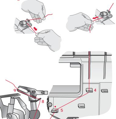
• Thread the looper area of the machine following the red color coded thread guides (4-9).
