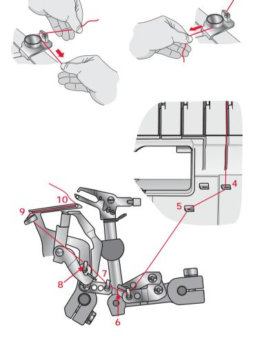
• To thread the last thread guide (9), pull about 10 cm (4") of thread through the guide (8).
