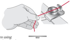
Note: When using decorative threads, place the thread unreeling disc as shown to prevent the thread from getting caught on the edge of the spool.
