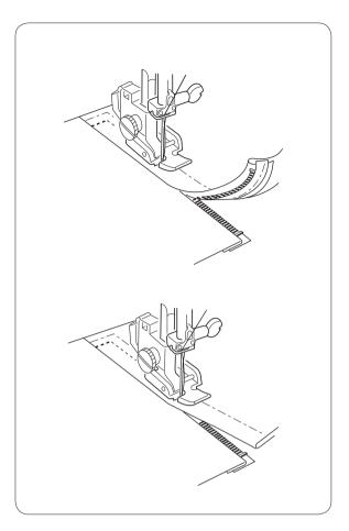
Move the zipper foot to the left pin. Guide the edge of the foot along the zipper teeth and stitch through garment and zipper tape. Stop about 5 cm  $(2^{\circ})$  from the top of the zipper.
