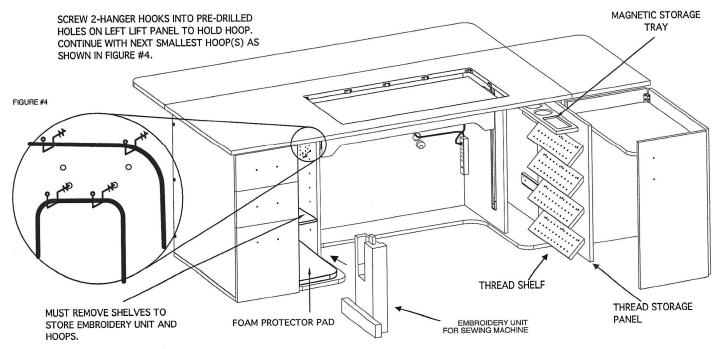
MODEL: 18A ELECTRIC LIFT PARTS DRAWING
