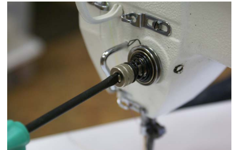
Figure 3-110 For fine adjustment of check spring insert screwdriver turn clockwise for more tension
