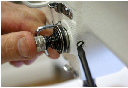
Figure 3-108 Tighten screw on your machine
