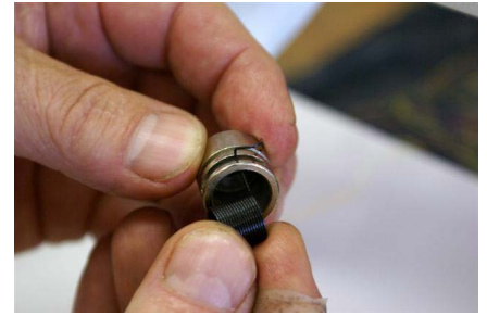
Figure 3-98 Twist while inserting the new spring
