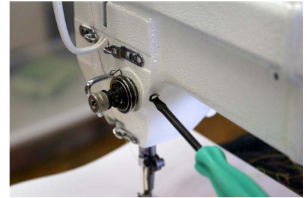
Figure 3-86 Screw on inside of machine loosen only. DO NOT REMOVE
