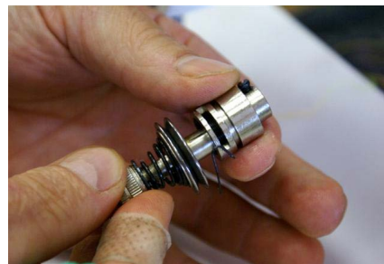
Figure 3-91 Remove tension assembly from barrel
