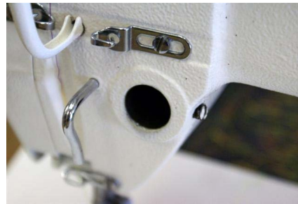
Figure 3-88 Machine with tension assembly re- moved
