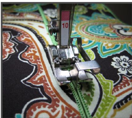
Create rolled edge seams by finishing single edges, placing them side-by-side, & stitching them together using matching or monofilament thread with a zigzag stitch.
