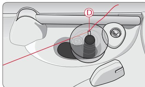
*Note: When using an earlier version of HUSQVARNA VIKING® bobbins that do not have a hole, wind several turns of thread on the bobbin to get started.*
