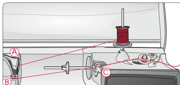
*Note: Depending on the type of thread, wrap the thread one or two turns around the bobbin thread tension disc (B) to put more tension on the thread.*
