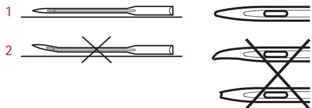
*Note: Change the needle often. Always use a straight needle with a sharp point (1). A damaged needle (2) can cause skipped stitches, breakage of needles or snapping of thread. A damaged needle can also damage the stitch plate.*
