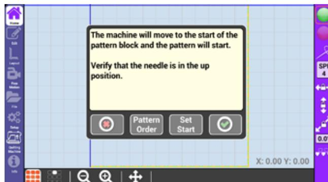
Set Start allows you to set the start position on the pattern. This is useful if you need to resume a pattern that has only been partially stitched, such as a pattern that had a thread break.
