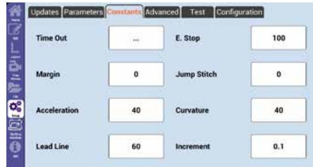
Increasing Acceleration increases the maximum acceleration and deceleration rate, while decreasing the Acceleration decreases the maximum acceleration/ deceleration rate.
