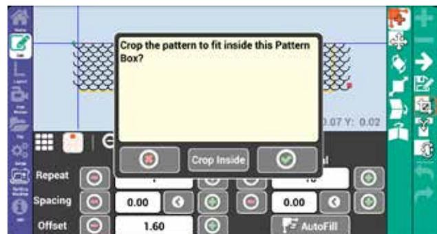
16. Press the offset green plus
