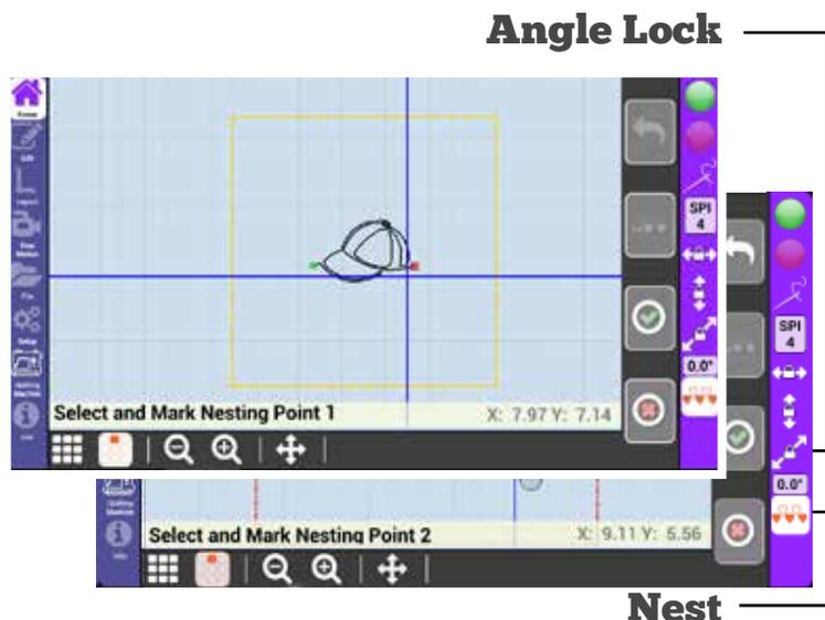
4. Once the quilt is rolled, follow the on-screen instructions to realign your machine with both the left and right marks created in step 1 and 2, and press the green check mark. (If you press the check mark at the incorrect point, use the undo button to try again.)
