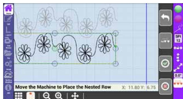
12. Move the machine to the first nesting point, press the green checkmark
