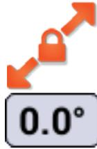
Angle lock allows you to set any angle, out of 360 degrees, that you would like to lock the machine.
