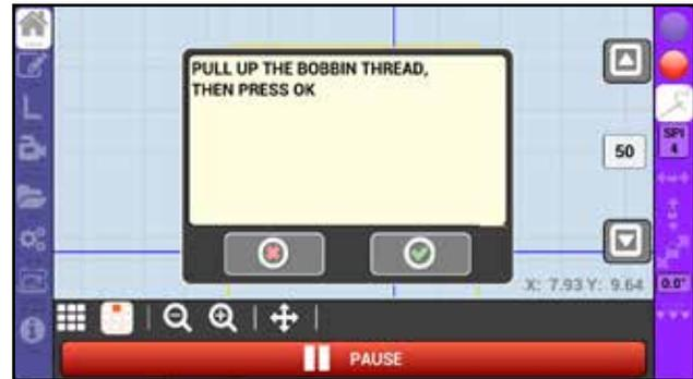
While the machine is following the pattern, you can adjust the speed by using the up and down arrows on the right of the screen. The lower the speed, the slower the system will move. (The speed defaults to the max speed settings in the Setup Parameters tab.)
