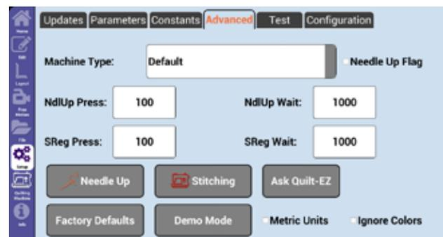
Machine Type must be changed from Default if Handle Bar connections are used. If not using handle bra connections, Default or a custom mode should be selected.
