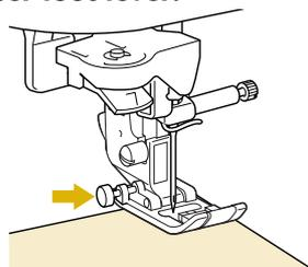
\* The presser foot remains level, enabling the fabric to be fed. Once the trouble spot has been sewn, the presser foot will return to its normal operation.
