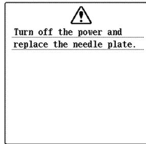
This message is displayed when you try to sew with a stitch other than a middle needle position stitch while the single-hole needle plate is installed. This message is displayed when the needle plate is removed with the machine on or when the machine is turned on in the embroidery or embroidery edit mode.
