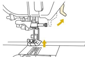
**4** Press the black button on the presser foot holder to remove the presser foot.
