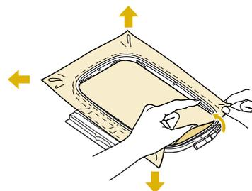
\* Make sure that the edges of the inner and outer frames are aligned.
