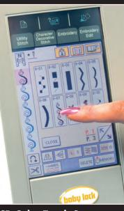
LCD Color Touch Screen (240 x 320 size) with touch pen This easy-to-read touch screen makes changing your machine's settings simple, and the color LCD screen allows you to edit your designs while distinguishing between thread colors.
