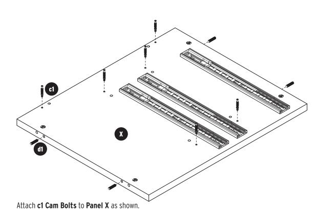
Insert d1 Dowel Pins into the edges of Panel X as shown.
