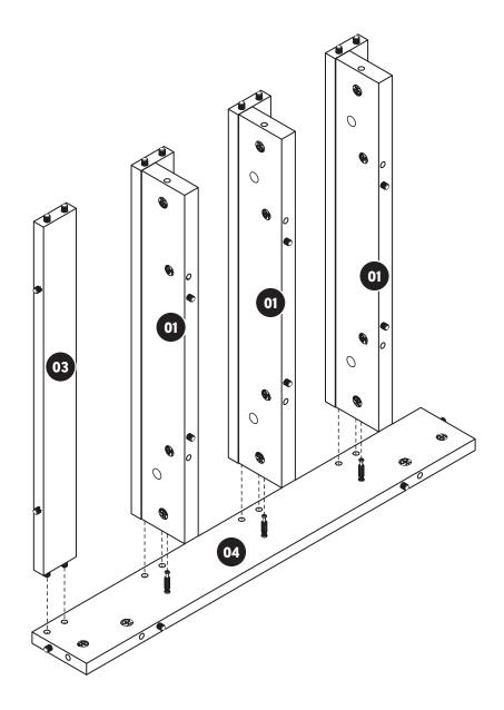
Attach **Panel 01/02** pieces to **Panel 04** by inserting cam bolts into cam locks. Tighten cam locks and apply **c2 Cam Covers.**
