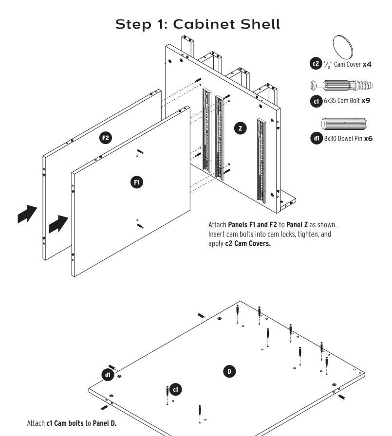
Insert d1 Dowel Pins into the edges
