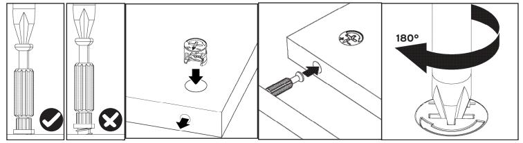
Screw cam bolts flush as illustrated.
