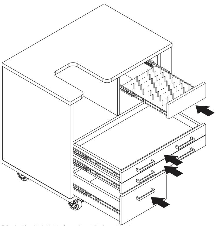
Fully extend the cabinet rails, align drawer rails, and slide drawers into caddy.
