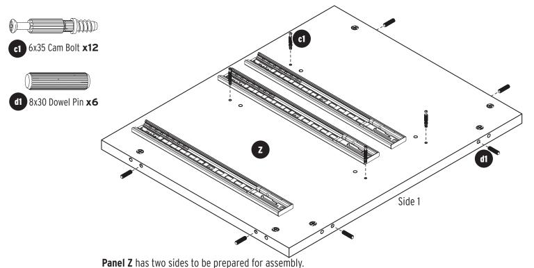
Prepare Side 1 of Panel Z with c1 Cam Bolts and d1 Dowel Pins as shown above.
