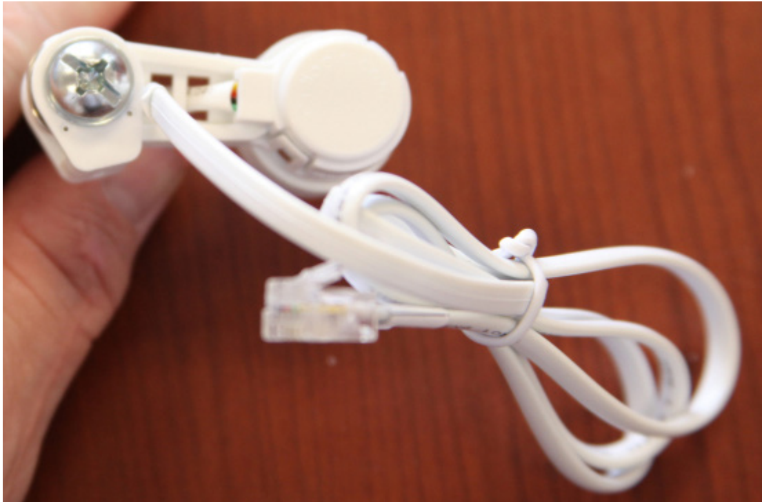
This shows the encoder without tension on the spring. Spring tab down between 5:00 and 6:00
