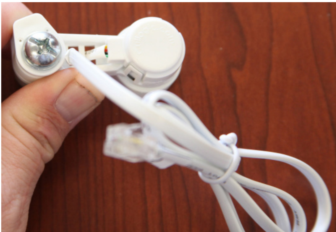
This shows the encoder with tension on the spring. When you have the encoder in place the Spring tab should be located between 11:00 and 12:00
